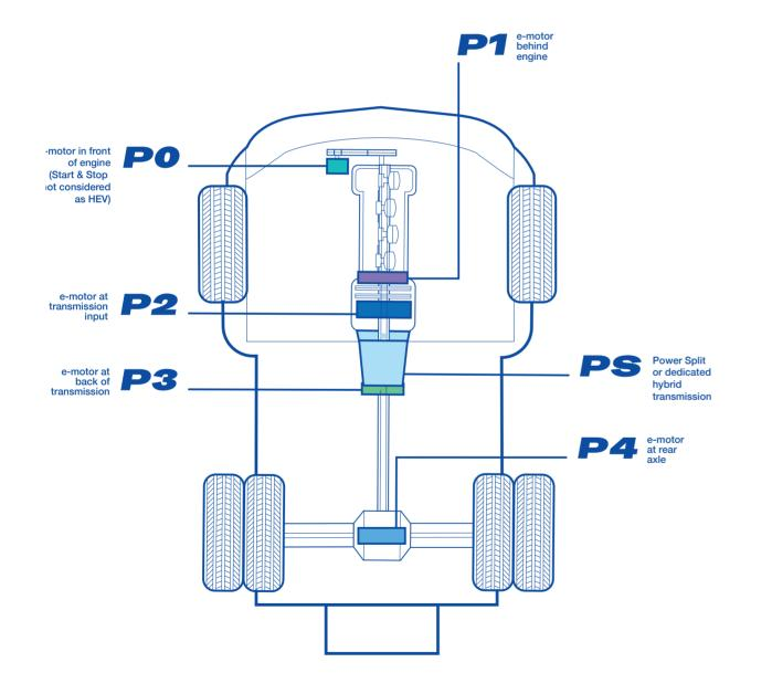
A Heavy-Duty Hybrid Vehicle is one of the solutions to reduce fuel consumption, improve efficiency and respond to climate issues for trucks, buses and off-road vehicles. The Heavy-Duty Hybrid Vehicle is equipped with an Internal Combustion Engine (ICE) and one or several electric motor. Two different sources of energy can be used: fuel and/or electricity.
